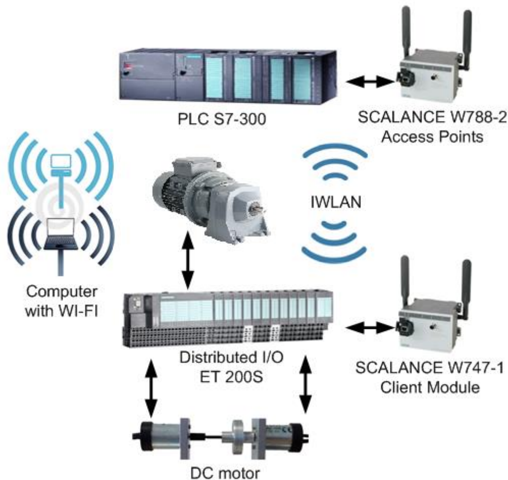
Figure 2-4: IWLAN system configuration
