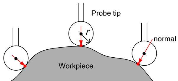
**Figure 10.** The radius compensation of CMM measurement
