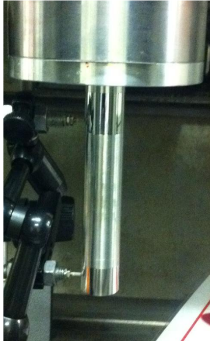
Figure 4.3 – Long Test-bar measuring tilt error motion
