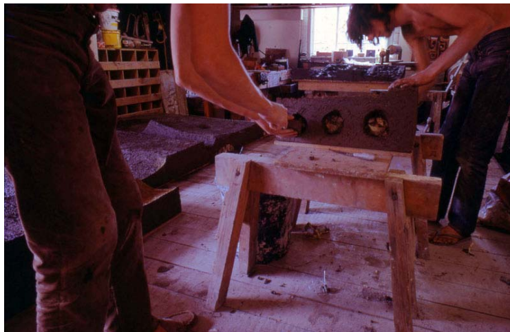
Figure 9-12 Cutting out surplus clay from a leather-dry Articulation in movement tile (Courtesy Fritz Steller)
