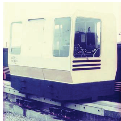
Figure 4. Low-speed 3.2 tonne Maglev vehicle
