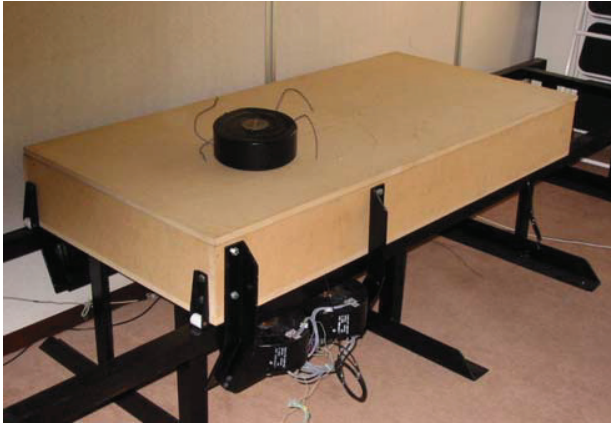
Figure 5. 200kg Maglev demonstrator vehicle
