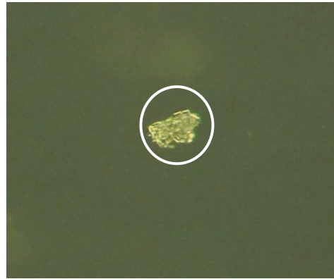
Fig (5) Optical Microscopy image “pit type defect”
