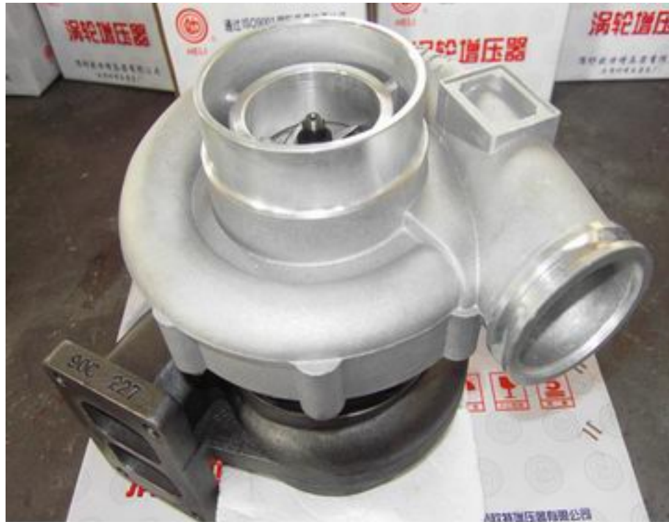
Figure 7. 2. The GJ90C turbocharger
