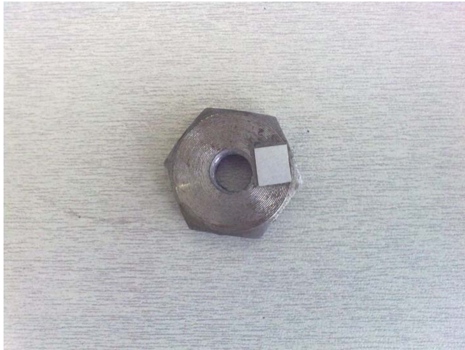
Figure 7. 10. The speed nut for the light sensitive belt placement
