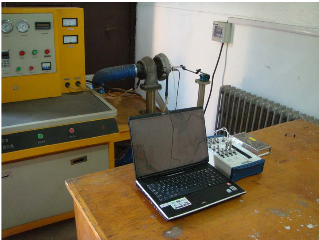
Figure 7. 13. A photograph of the turbocharger test rig
