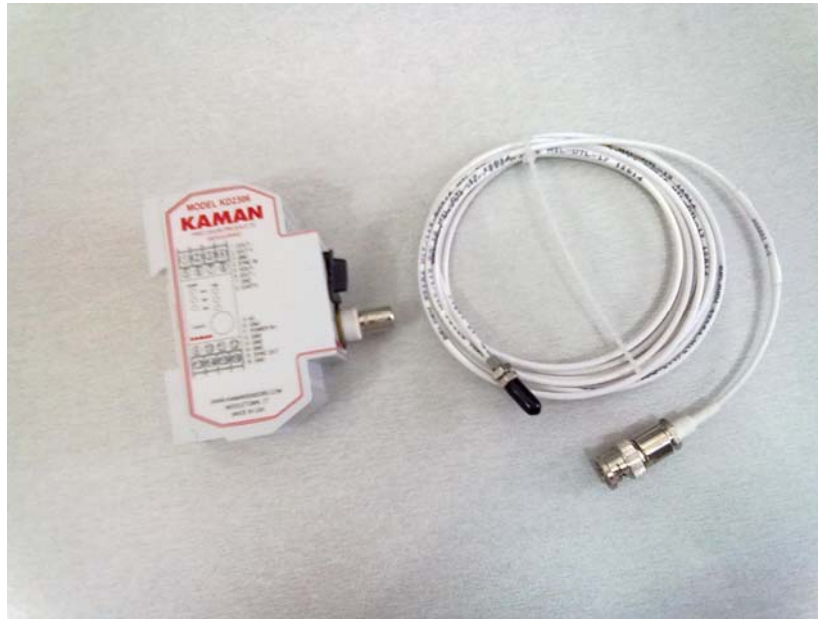
Figure 7. 7. KAMAN KD2306 1U1 eddy current displacement transducer
