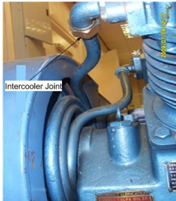
**Figure B-3 Intercooler leakage**
