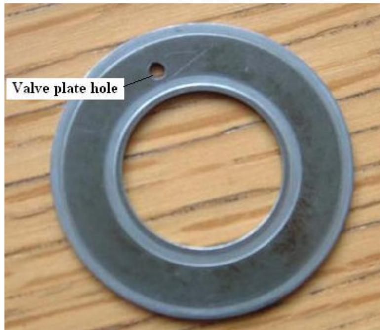
**Figure B-2 Leakage in second stage valve plate**
