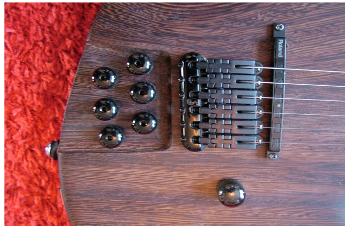
Figure: 46 GK3 pickup installed
