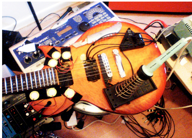
Figure: 21 installing piezo pick-ups
