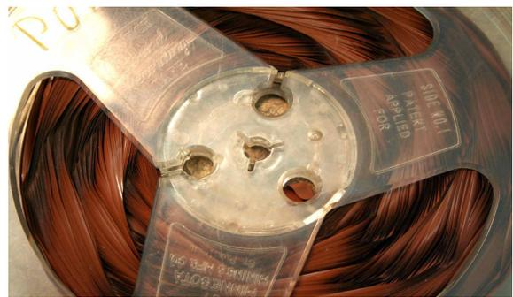
Fig.1: a tape affected by severe curly deformation.
