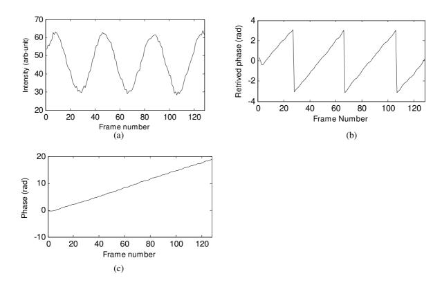
Fig. 2. Measured Interference fringe and retrived phase distribution (a) intensity distribution of 128 frames for one pixel (b) retrived phase discontinuity distribution (c) phase continuity distribution.
