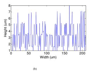
Fig. 5. Measurement result of semiconductor daughterboard sample with a sinusoidal mechanical disturbance of 40 Hz and 400nm peak to peak. (a) measured surface and (b) cross-sectional profile.
