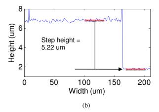
Fig. 6. Measurement result of semiconductor daughterboard sample with vibration compensation. (a) measured surface and (b) cross-sectional profile.
