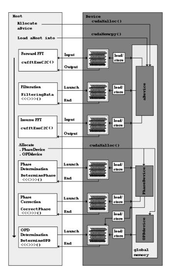
Fig. 7. The proposed CUDA program structure.
