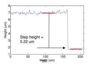
Fig. 4. Measurement result of semiconductor daughterboard sample without an induced mechanical disturbance. (a) measured surface and (b) cross-sectional profile.
