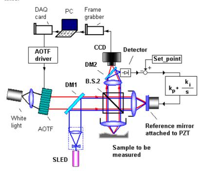
Fig. 3. Stabilised WSI interferometer
