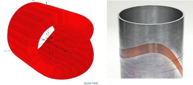
Figure 5: A multipole helical coil (left) and test winding (right)
