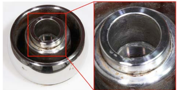
Figure 1: Photographs showing a case of severe taper corrosion with imprinting of the stem taper screw thread onto the head taper surface
