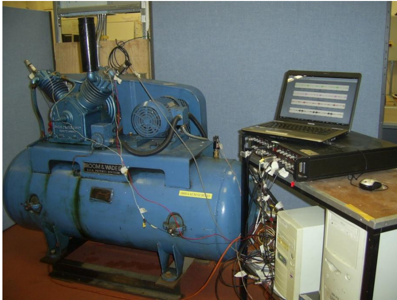
Figure 1. Reciprocating compressor test system.
