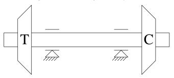
Figure 2(a). Physical model of turbocharger rotor system.
