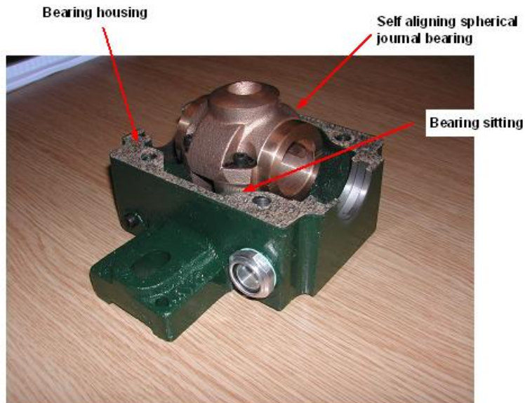
Figure 1. Self-aligning spherical journal bearing components
