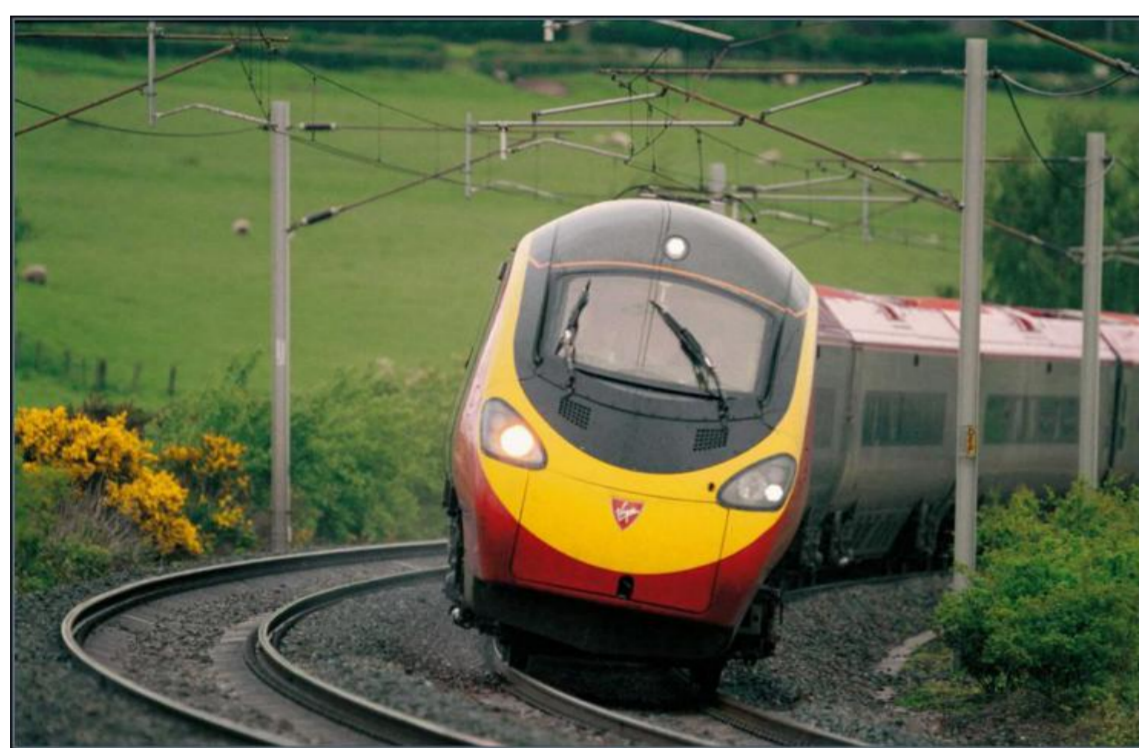
Tilting technology on a pendolino train (Source: Virgin website)
