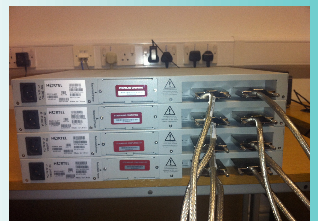
Nortel 5510-T switches for Sol cluster with interconnects
