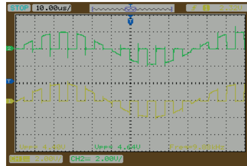
FIGURE 5. the excitation signals in array A and B
