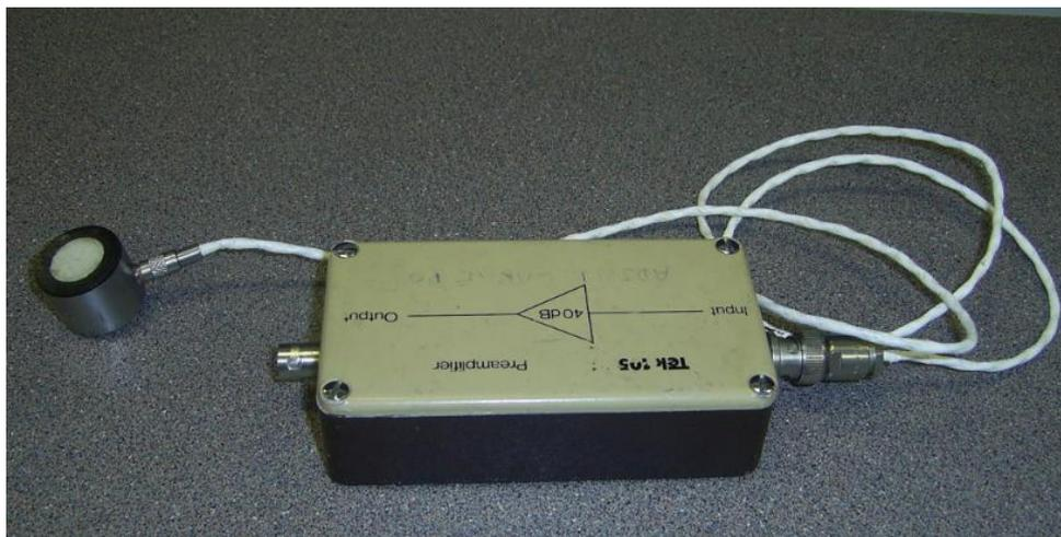
**Figure 4- Acoustic Emission Transducer**
