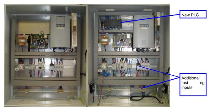
Figure B-3 - Test rig panel interior before and after modification
