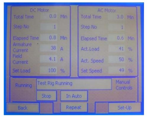
Figure C-23 - Operator Screen; Test Rig running in Auto
