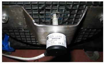
Figure 7-2 - Mounting of motor encoder
