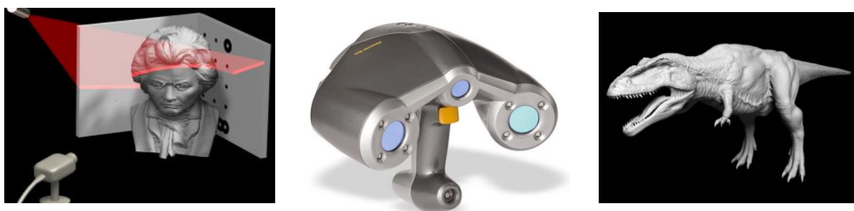
Fig 22 – Scan in progress, hand held device and similar detailed output
