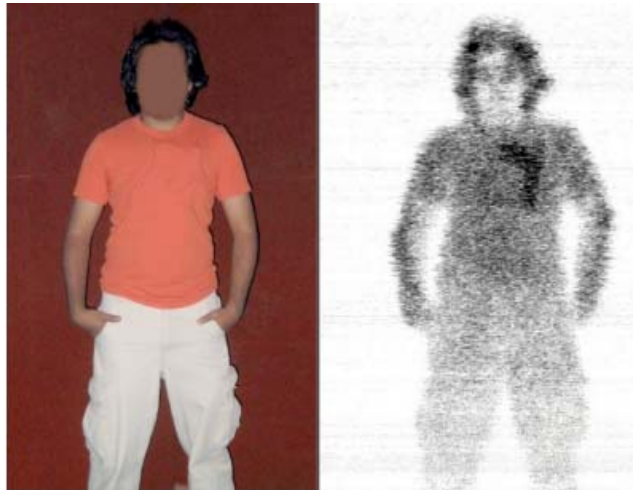
Figure 2.10. THz reflection image of a person carrying a gun [26].
