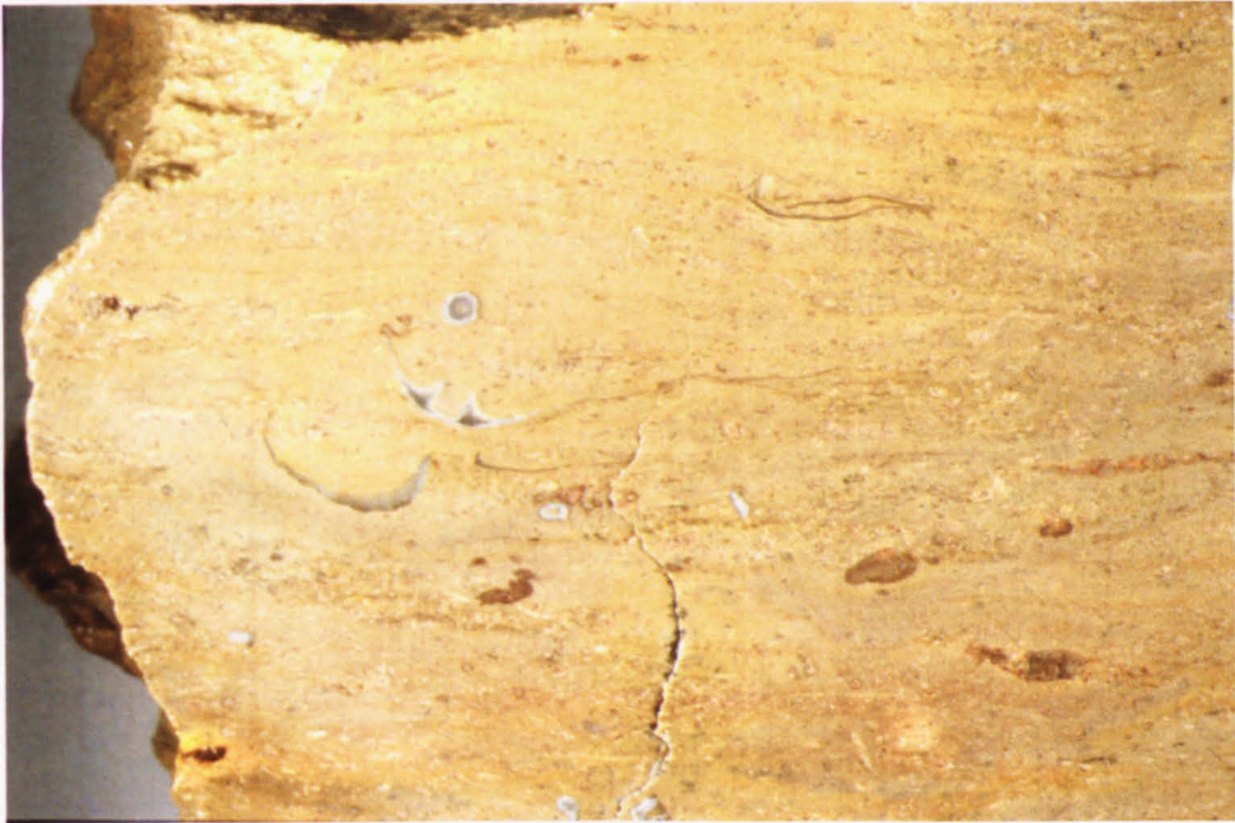
Plate 11. Sample of intramound horizon taken from Skreen Hill I of Marble Arch Cave, showing the relative abundance of shell fragments and ferric iron. (John Gunn).
