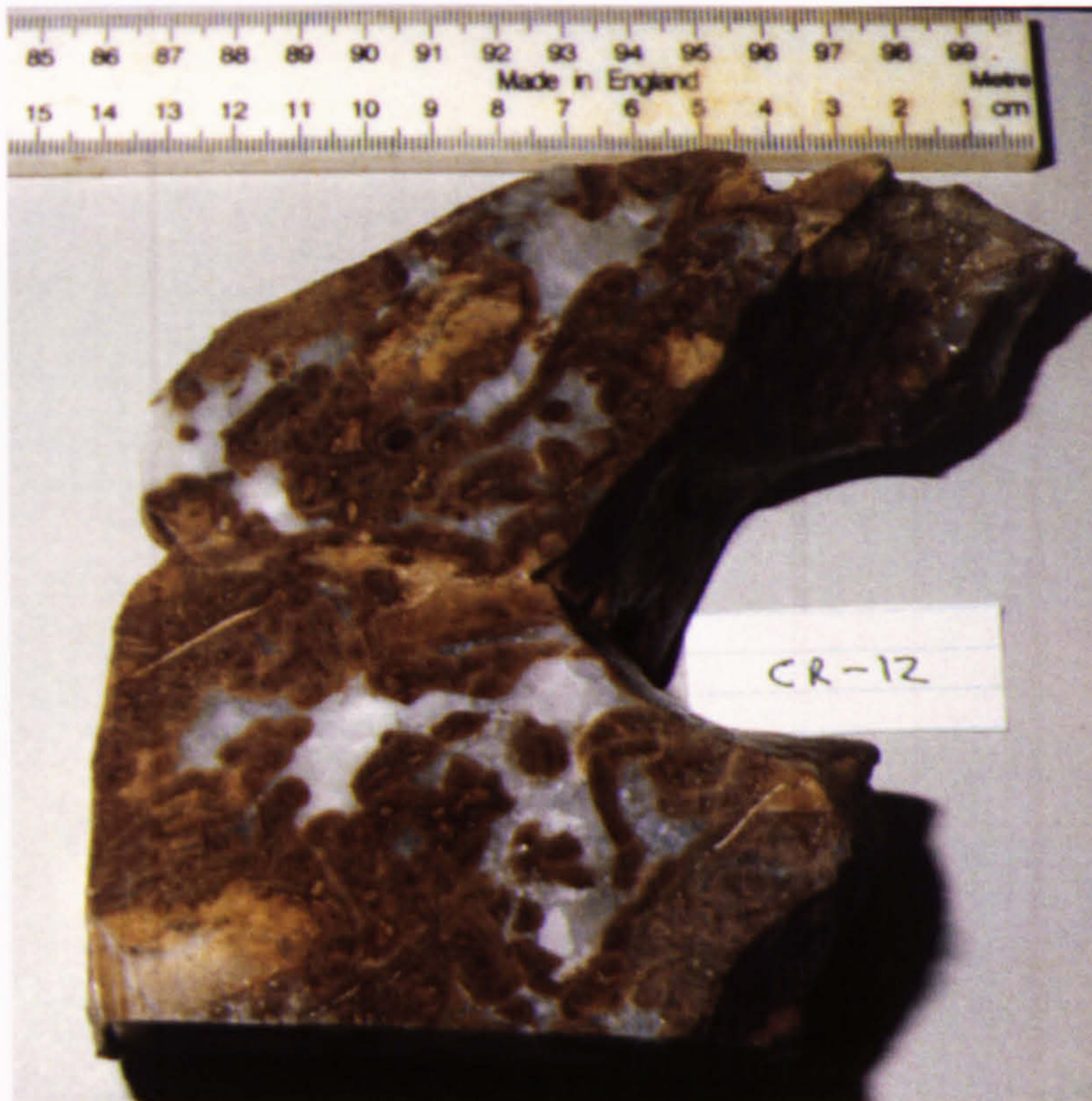
Plate 12. The stromatolite structure commonly found within the vertical-type mud mounds. Showing shelter cavities associated with bryozoa and final stage blocky calcite spar. (John Gunn).
