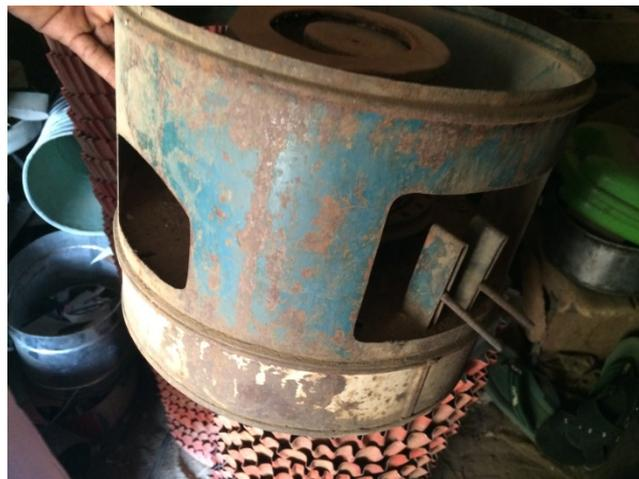
**Figure 28: Kerosene stove partly made from salvaged aluminium roofing sheet**
