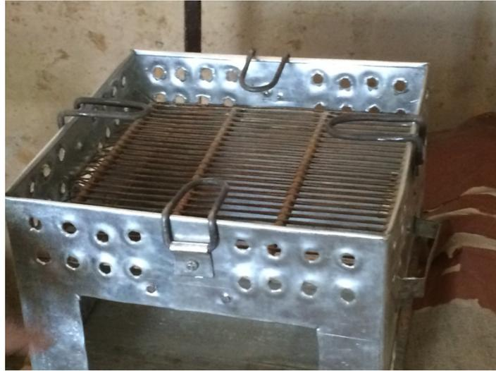
**Figure 29: Coal stove made from combination of salvaged roofing sheets**
