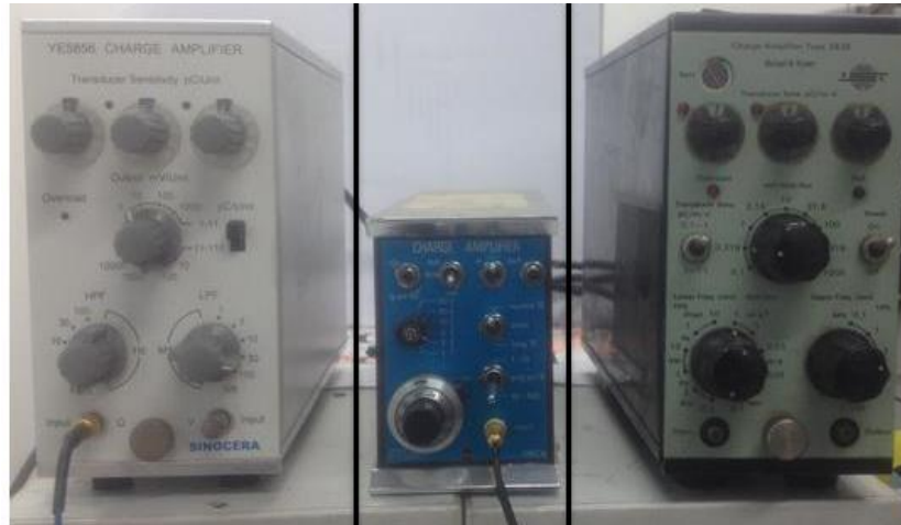
Figure 6-11 Charge amplifier set to collecting data
