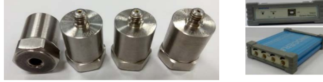
(a) Acceleration Sensors (b) Data Acquisition
