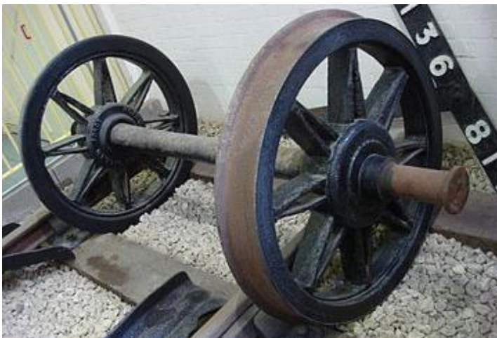
William Jessop's flanged Wheelset and Fish-belly Edge Rails circa 1806
