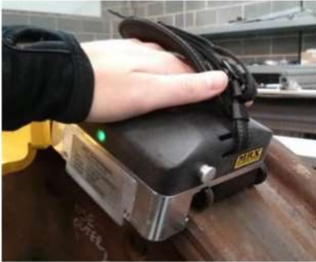
Figure 3. Wheel surface crack measurement hand-held unit and sensor array
