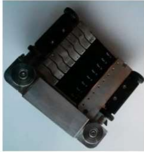
Figure 3. Wheel surface crack measurement hand-held unit and sensor array
