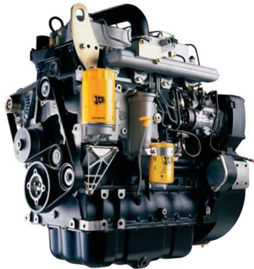
Figure 4.2 The JCB444 TCA 74kW diesel engine
