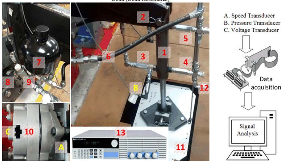
Figure 3. Key components of regenerative shock absorber system.
