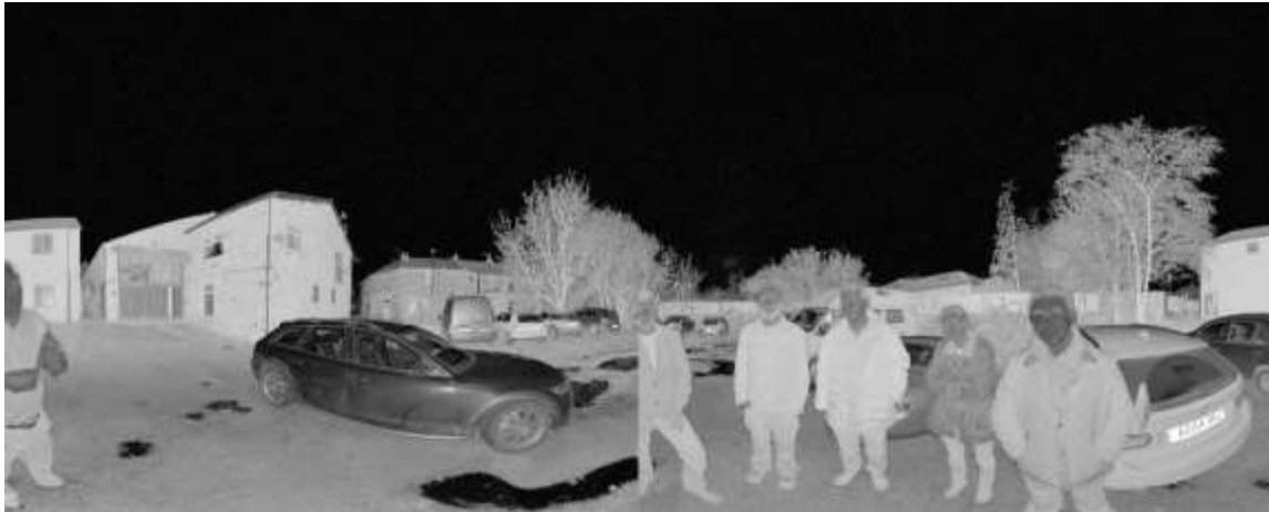
Figure 32: Faro X30 point cloud 3D data.
