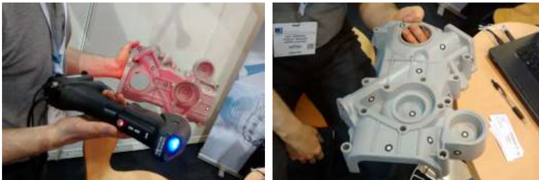
Figure 11: Creaform 300 demo showing high tolerance measurements
