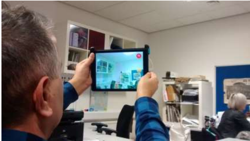
Figure 17: 3D scanning an office with SDK Structure Sensor connected to iPad
