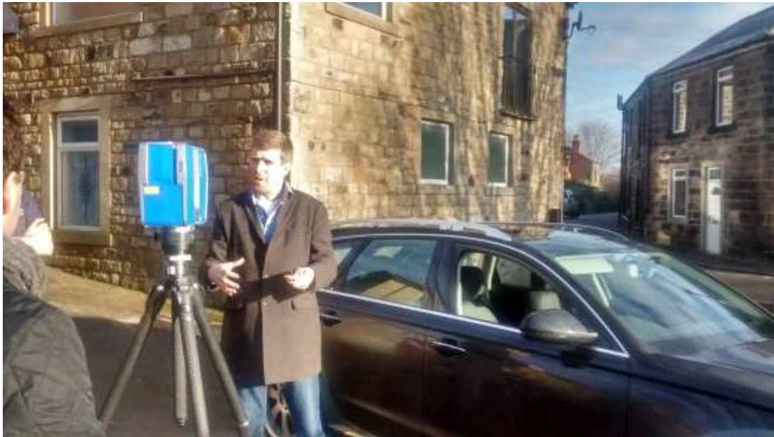
Figure 30: Faro scanning setup
