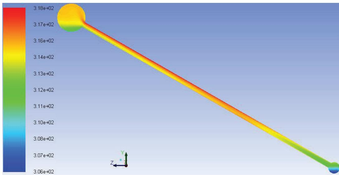
Figure 3 Temperature variations within the thermo-syphon after 1 hour of operation
