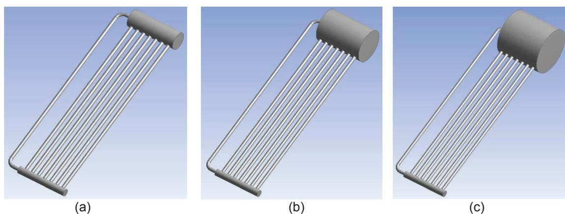
Figure 1. Thermo-syphon models having condenser diameter equal to (a)  $5 * d$  (b)  $10 * d$  and (c)  $15 * d$
