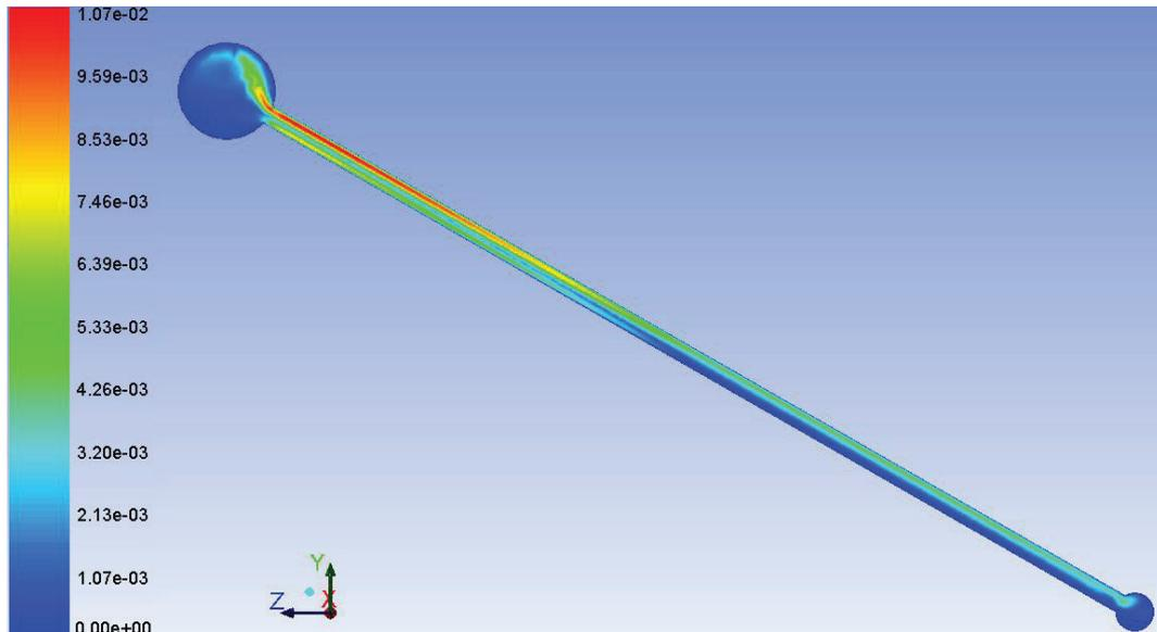
Figure 2. Velocity variations within the thermo-syphon after 1 hour of operation
