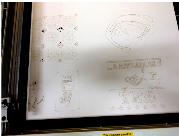
Figure 9. Examples of student's digital drawings hatched and cut onto paper using the laser cutter
