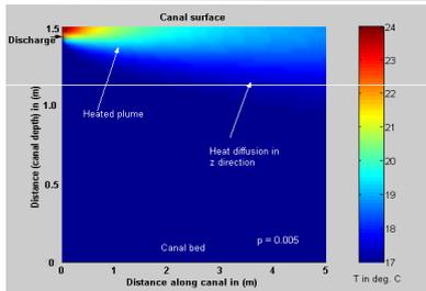
Model applied on Matlab shows temperature distribution profile through the depth
