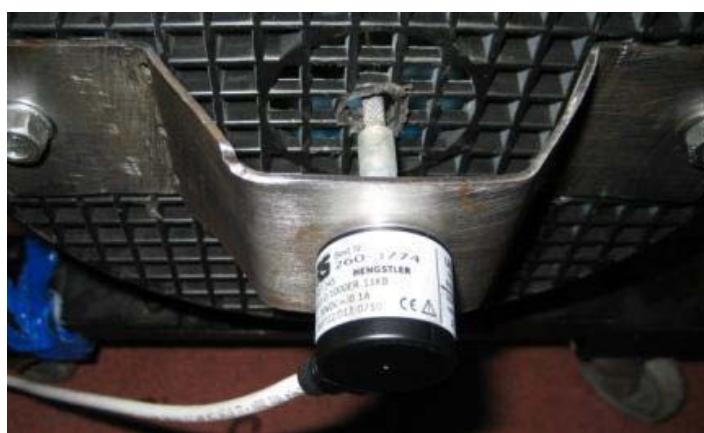
**Figure 7-2 - Mounting of motor encoder**
