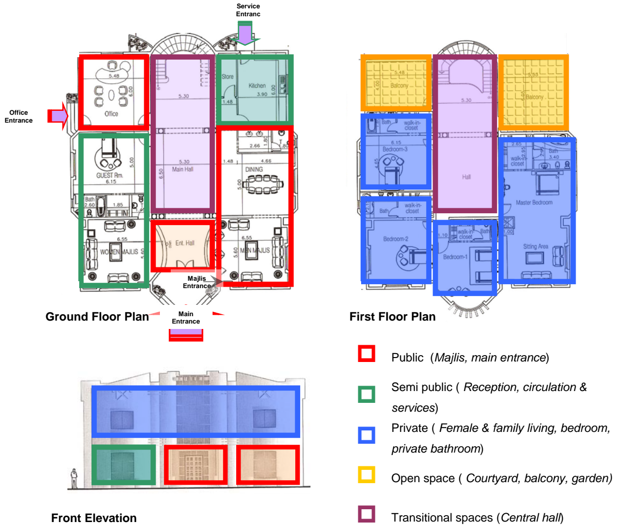
Figure 6.36. -Schematic analysis for space organization in a contemporary house in the UAE (Source: the author)
