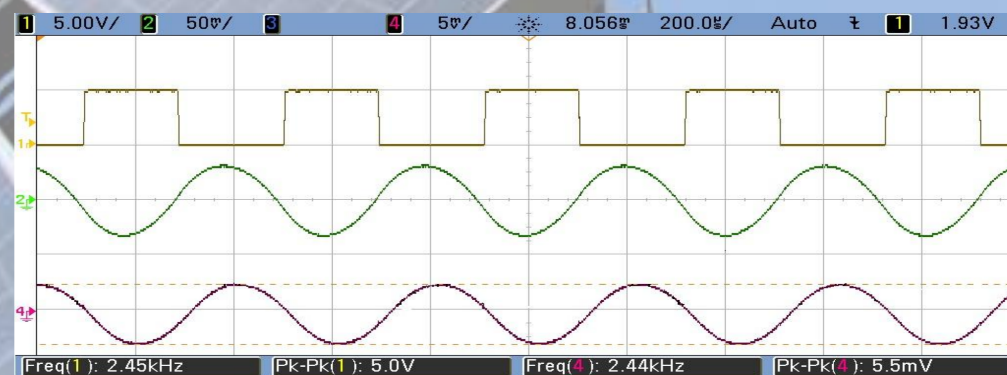
Fig. 3 Current Ripple for a 50% Duty Cycle (2.5A) Represented on Channel 4, 1mV = 10mA.
