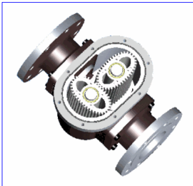
Figure 2.9 Chambers in positive displacement meter (Yeung, 2003)
