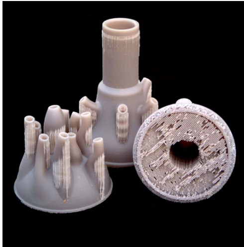
Figure 84 Thermojet Wax Patterns
