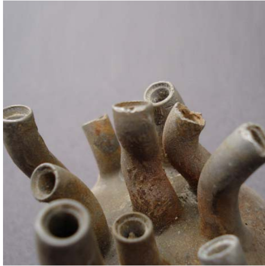
Figure 81 Casting Problems at the Tentacle Tips
