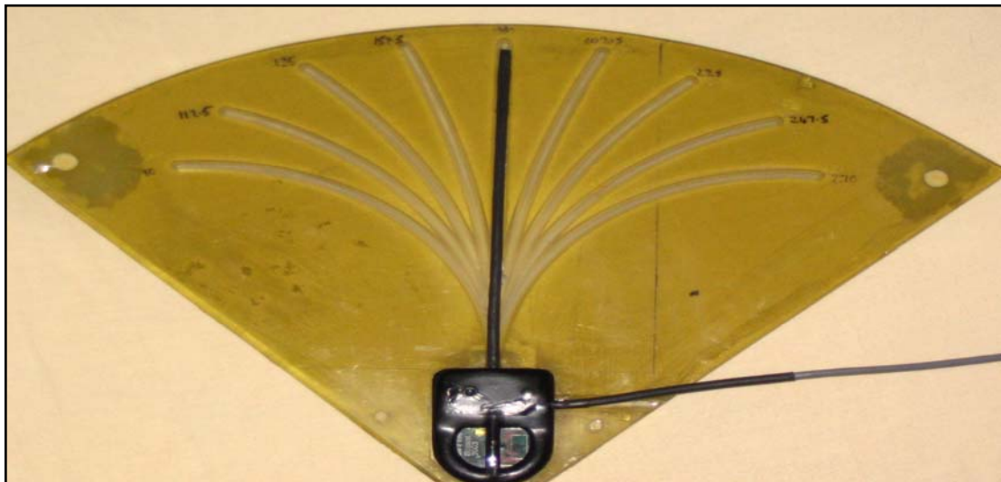
Figure 8: The modified slotted calibration jig containing a hip FOG
