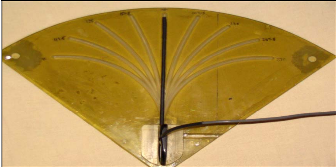
Figure 7: The modified slotted calibration jig containing a lumbar FOG
