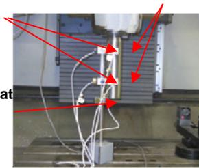
Figure 4: NCDTs located around on the the tool
