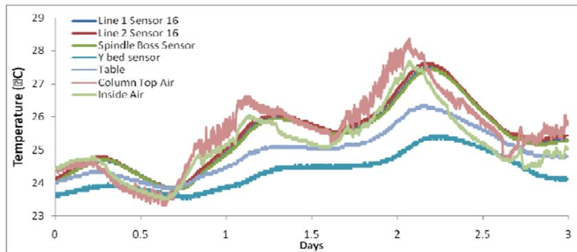
Figure 13: Environmental temperature variations recorded over 3 days
