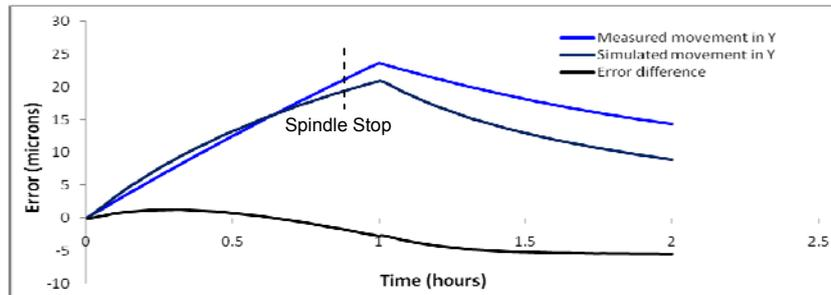
Figure 8: Correlation plot of the experimental and simulated displacement profiles
