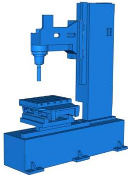
Figure 1: Full machine CAD model created in ABAQUS 6.7-1
