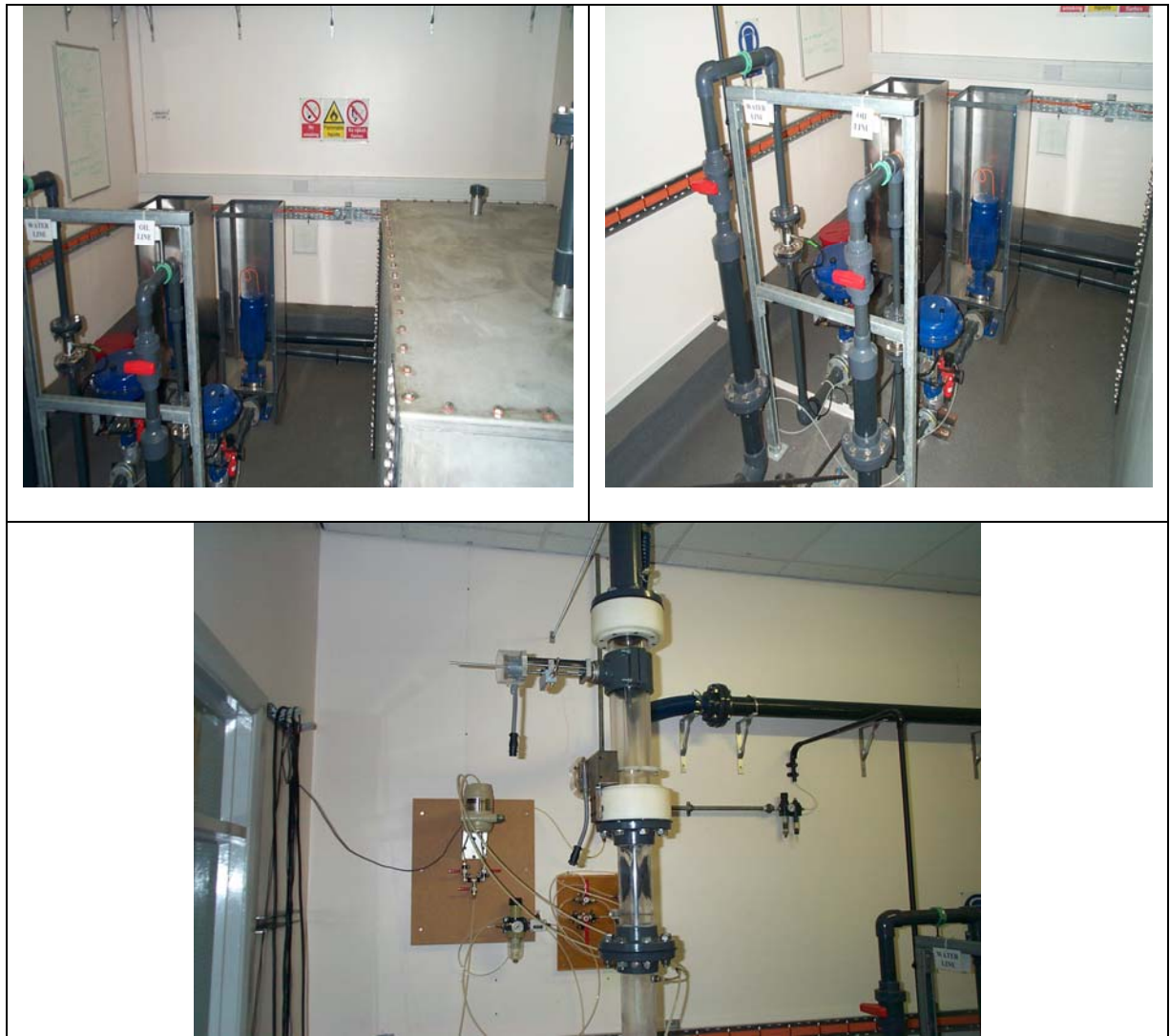
Figure 25. The oil-water loop. The tank and the pumps (top-left), the pumps the valves and the turbine meters (top-right), and the working section (bottom).
