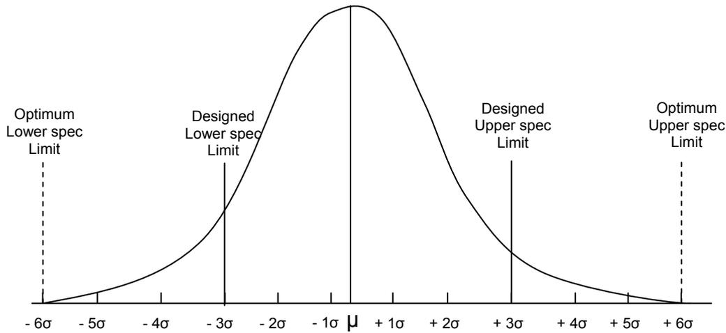
**Figure 1 – Normal Distribution, 3 sigma design, 6 sigma optimum design**
