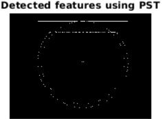
Figure 4.18: Edge detection using phase stretch transformation
