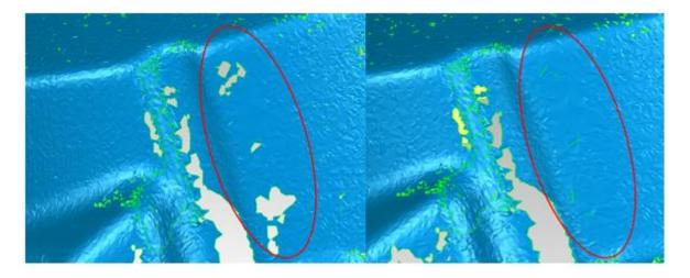
Figure 3.6: An indication of how the flat hole-filling technique is performed
