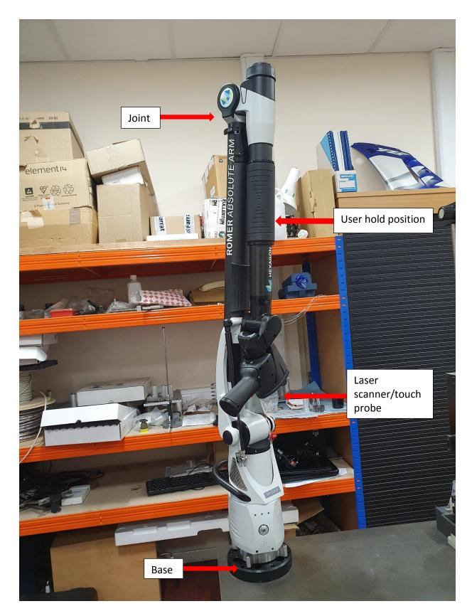
Figure 2.14: Articulated Arm CMM (AACMM) with an attached laser scanner and a magnetic base for minimising vibration
