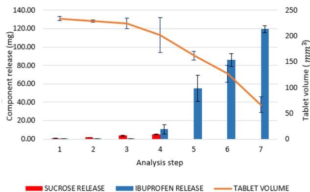
**Figure 1.** Correlation between tablet volume and release of sucrose and ibuprofen after each experimental step.
