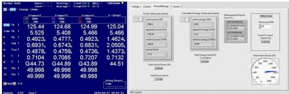
These analyser displays cannot be directly compared as they have largely different applications. The LabVIEW-based analyser was designed for use in small monitoring, recording or setup applications, to name a few, and therefore requires a more user-friendly, softer-looking display than the industrial, clinical appearance of the more portable Yokogawa unit.
