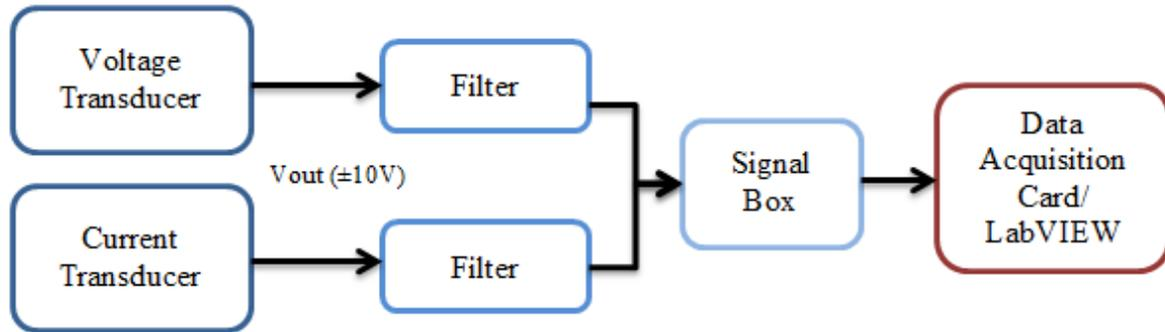
The final analyser was tested on a 5.5A, 220V-rated AC induction motor, giving a per-phase voltage of 127V (rms), which was specified as the upper per-phase measurement value (before headroom) of the analyser electronics.
