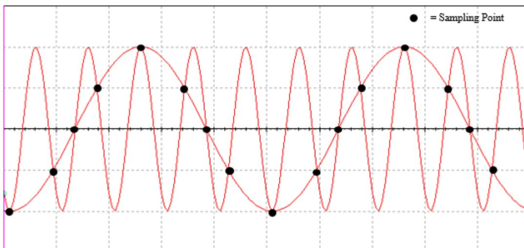
To avoid this under-sampling, the Nyquist sampling limit is a well-practised method that ensures that a signal is properly measured and reconstructed. It states that a signal should be sampled at a minimum of twice its own frequency, but often, in practice, it is usually higher, to reduce the filtering requirements and provide a more detailed measurement of the signal if possible.
