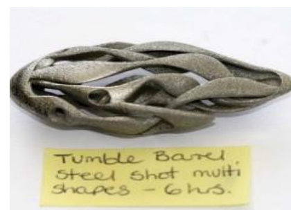
Figure 211 Conventional Polishing – Steel Shot
