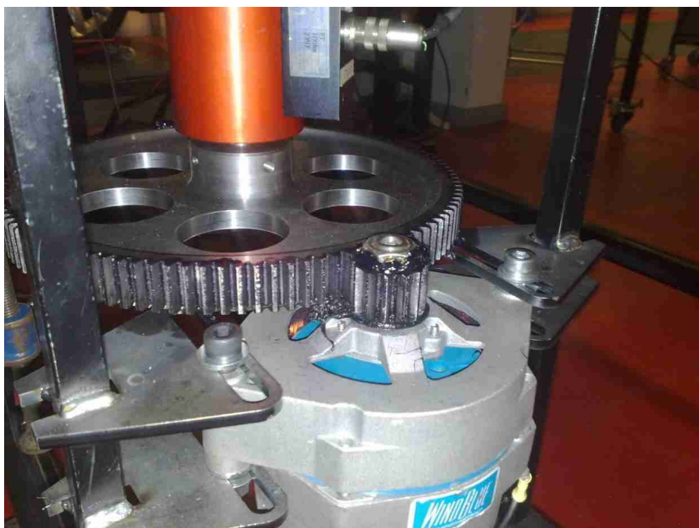
Figure 4.2: Torque transducer, gear train and generator
