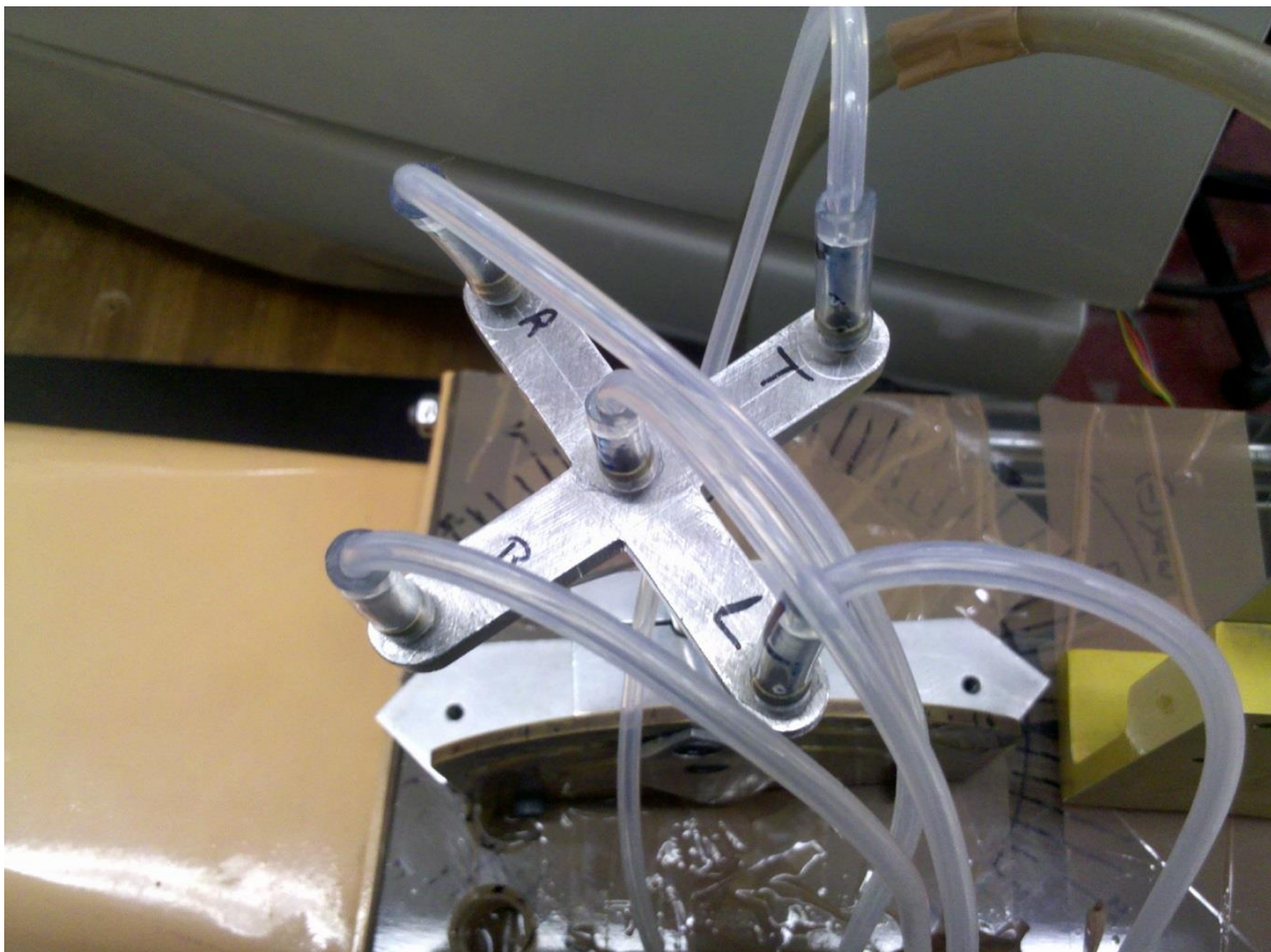
Figure 3-8: Five hole probe mounted on the traverse in the wind tunnel
